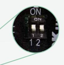
Switch 1 allows the minimum brightness to be adjusted
