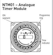
**Time control segments:** 1 segment = 15 minutes, push segment down for ON, pull up for OFF.
