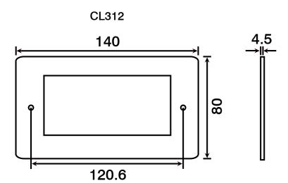
Errors & Omissions excluded. Specification is subject to change without notice. All Metal Clad New Media modular plates are provided with 40mm deep back boxes.
