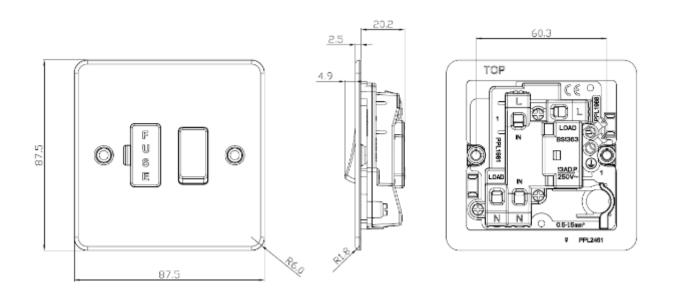
Fused spur units or connection units are an electrical switch with a built in fuse, designed for appliances that do not have or require a fused plug top. Fused spur units are also used for high powered electrical equipment with heavy continuous load, so that the appliance can be isolated by a single cable from a ring main for safety and maintenance purposes. 13A rated available with and without a double pole switch, neon and flex outlet.
