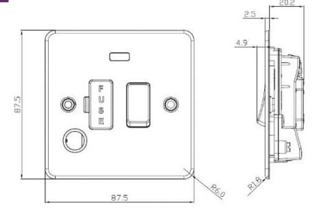
Fused spur units or connection units are an electrical switch with a built in fuse, designed for appliances that do not have or require a fused plug top. Fused spur units are also used for high powered electrical equipment with heavy continuous load, so that the appliance can be isolated by a single cable from a ring main for safety and maintenance purposes. 13A rated available with and without a double pole switch, neon and flex outlet.
