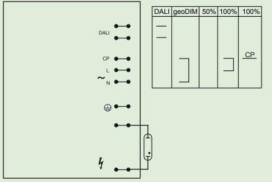
CP= Control Phase Where a DALI command is detected, DALI dominates over all other dimming methods.
