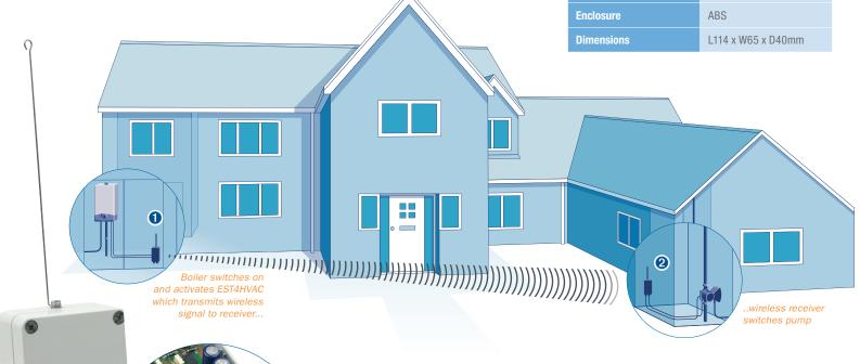
With four inputs this product is designed to work with the EasySwitch single circuit (ESR.1) or four circuit (ESR.4) receivers to allow remote switching of up to four electrical circuits within a building or from one building to another.
