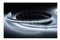
This specialised strip utilises very small LEDs (20:16) arranged in a close formation that effectively eliminates the visible shadow present in many LED strips. This creates the effect of one continuous line of light, particularly when installed within an aluminium profile. The Spotless strip also has a high colour rendering index of CRI 90 and is very bright at 1550 lm/M, which means the strip can be used to create custom luminaires.
