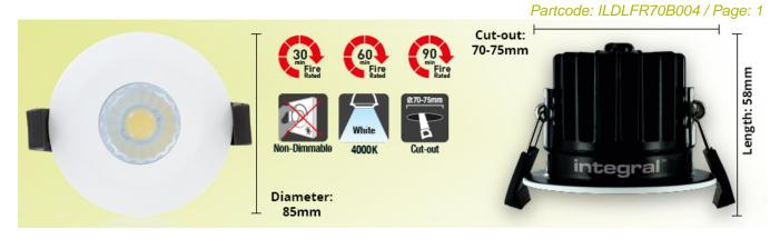
These low-profile lamps are fire rated to 30, 60 and 90 minutes, Air Tightness compliant with Part C and Part L and Resistance to Sound compliant with Part E. Warm White and Cool White colour temperature options and dimmable or non-dimmable options are available. Importantly, these lamps are IP65 rated and designed to offer the safety and quality of other Fire Rated Downlights but with a lower price-tag.
