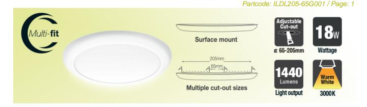
This ultra-thin (15.5mm) downlight is supplied with configurable brackets and clips allowing for installation in a cut-out from 65-205mm as well as having a surface mount installation option. Visible flicker is eliminated with the integrated driver and a frosted diffuser provides uniform light.
