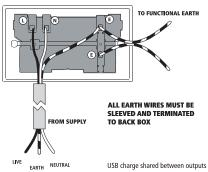
2 gang Unswitched Socket Line Drawing Connect the cables as shown in the diagram.
